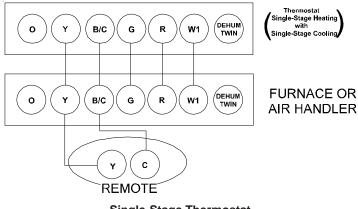
Single-Stage Thermostat with Two Low Voltage Wires to Remote
